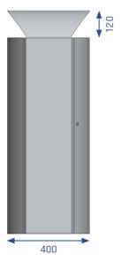
**Description:** Self-supporting, curved stainless steel outer walls, connected to stable flat side panels. Curved door with recessed lock (a key is supplied with each container). The door retention profile prevents the hinges from overstretching. A curved cover is firmly connected to the structure. The shape of the cover results in reduced height from two sides. A sturdy insertion ring guides waste into the waste bag.
