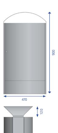
**Description:** Self-supporting, curved stainless steel outer walls, connected to stable flat side panels. Curved door with recessed lock (a key is supplied with each container). The door retention profile prevents the hinges from overstretching. A curved cover is firmly connected to the structure. The shape of the cover results in reduced height from two sides. A sturdy insertion ring guides waste into the inner liner.
