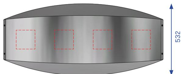
**Description:** Self-supporting, curved fronts and flat side panels made of stainless steel, secured with an internal construction of galvanized steel, provide great stability. The tops funnel-shaped openings guide waste into the inner liners and are also an elementary part of the fire protection (patented and certified).
